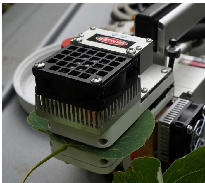
Figure 3: LICOR 6400 portable photosynthesis system IRGA chamber with leaf.
