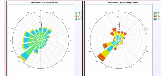
For example, the wind roses above show frequency of wind speed (left) and max wind speed (gust, right) at New Brunswick, NJ, based on hourly data from 2009 to 2011. There appears to be a clear dominance of Southwest winds on both charts, especially at slower wind speeds. More research is needed to determine whether this observed phenomena occurs naturally, or due to station siting or other factors.
